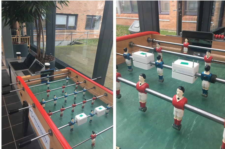
(a) Picture showing the football table setup with the computers receiving sensor data (b) Picture showing how two boxes are attached to a single handle to verify that the data we receive is consistent
